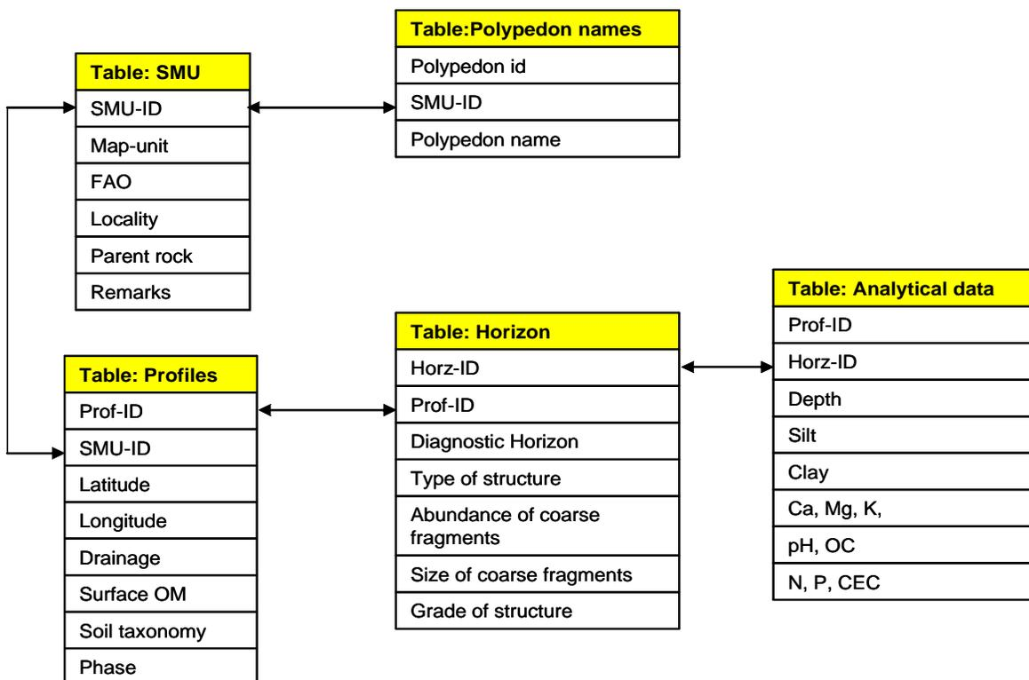
Figure 2. Structure of the SGDB at KARI
